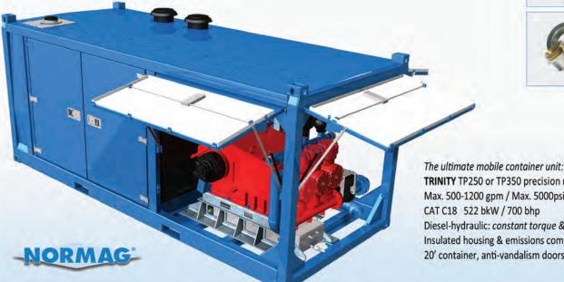
TRINITY TP250 or TP350 precision roller bearing pump Max. 500-1200 gpm / Max. 5000psi CAT C18 522 bkW / 700 bhp Diesel-hydraulic: constant torque & infinite speed control Insulated housing & emissions compliant 20' container, anti-vandalism doors
