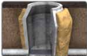
Grout curtain stops infiltration
