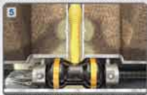
Lateral packer injecting grout
