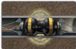
Chemical grout injected into soil
