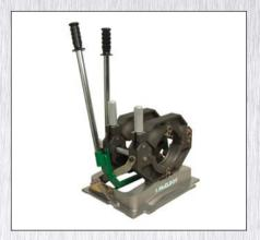
Centerline Guidance System, a semi-automatic locking cam system that maintains force during the cooling cycle and the ability to fit on the Manual Fusion Stand accessory. The 26 fusion unit has a greater mechanical advantage ratio to the popular 14 PitBull, as well as an electric facer with balance point handle for fast facing of pipe. Contractors and pipeliners that already own McElroy's PolyPorter and PolyHorse can enjoy the same productivity-enhancing benefits with the new 26 PitBull.
