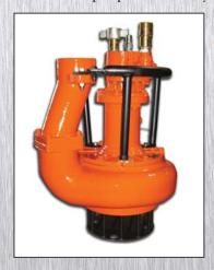
lic submersible line of pumps. Capable of flow rates to 1,000 gpm and heads to 170 ft, the HS103 is a compact, self-contained, hydraulic powered submersible pump with a diesel-driven hydraulic power unit. The HS103 is a cast-iron pump with cast chromium steel impeller designed for general pumping, slurries and sludges with solids handling to 3 in. in diameter, ideal for sewer bypass and municipal sludge applications. The unique top discharge design on the HS103
