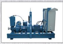
unlike most automatic priming systems, prevents product blow-by of pumpage, such as sewage, effluent and waste, from being discharged onto the ground or through hoses that carry the pumpage back to the source, making it environmental friendly. The durable construction and the highly efficient pump provides longer life and economical operations but most importantly - lower fuel costs. Consult Thompson Pump for options, accessories, applications assistance and alternatives.
