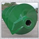
and larger on a retractable base. This innovative idea allows the cutting head to retract the outside gauge cutters to be extracted through the casing and reinstalled after inspection. The head expands to over cut 1-1/2 in. larger than the OD of the casing by turning it clockwise and retracts to 1-1/2 in. less than the OD of the casing by turning it counter clockwise for retrieval. With a patented duel-cam action the gauge cutters are mechanically opened and closed for positive engagement.
