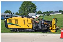
Deutz engine powers the machine and is capable of 12 percent greater power compared to its predecessor, the D16x20 Series II. The D20x22 S3 features 19,550 pounds of thrust/pullback with 2,250 ftlb of torque. The D20x22 S3 has a faster carriage speed, which can lead to an increased amount of product installed per minute. The 167 ft (50.9 m) per minute
