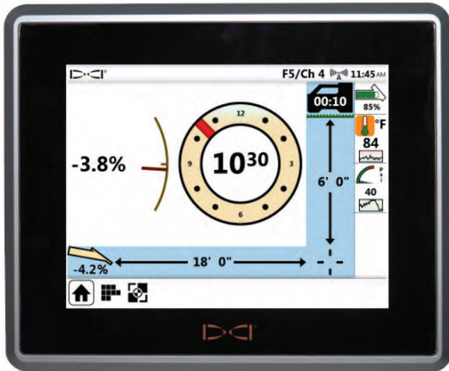
DCI's new remote display, the DigiTrak Aurora, is a 10-in. color touchscreen with wireless and Bluetooth connections. The concept of wireless delivery and the ability to add apps make the device easy to upgrade.
