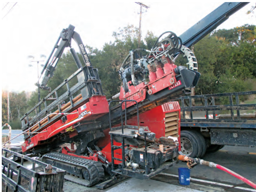
Accu-Bore pulled its 100,000-lb pullback JT100 working south of Los Angeles so it could be used on this crossing, 60 miles north of San Francisco.
